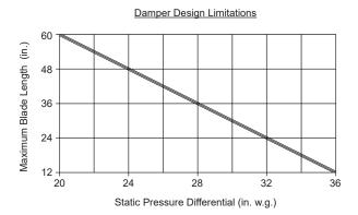
This damper's design at a blade length of 60" has a maximum allowable blade deflection of L / 360 for the static pressure indicated on the chart. At reduced blade lengths, higher static pressure limits can be attained without sacrificing damper operating performance characteristics.
